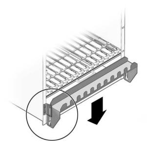
2. Disengage the injector/ejector mechanisms at the top and bottom of the blade server to notify software that the board is about to be removed. Wait for the Hot-Swap LED to light.
